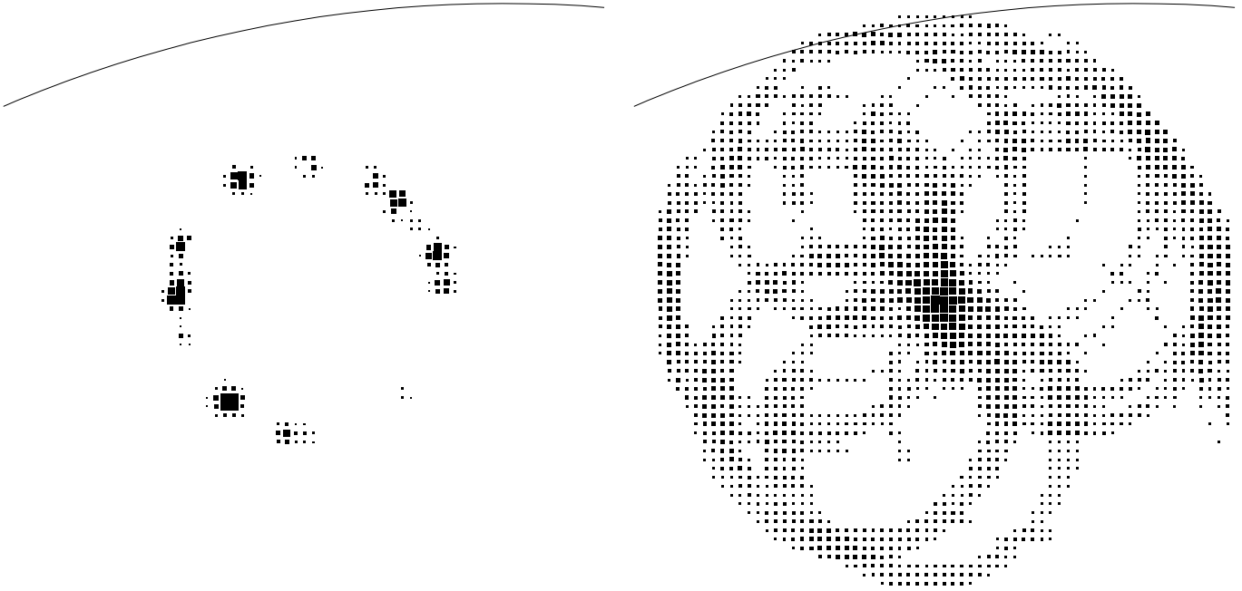
Fig. 4. Photon hits, registered by the electronic charge induced on the pad plane of the UV detector, form a Cherenkov ring of radius R (left). The Hough image of each photon hit is a circular band with Hough radius R_H of the mask, displayed in the correlation plane (right). For R_H = R , the images ideally would have one point in common, the center of the Cherenkov ring
